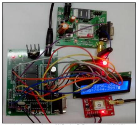
Hardware Interfacing of 8051 with GPS Receiver and GSM900
