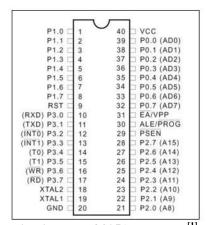
Pin diagram of 8051 controller<sup>[1]</sup>
